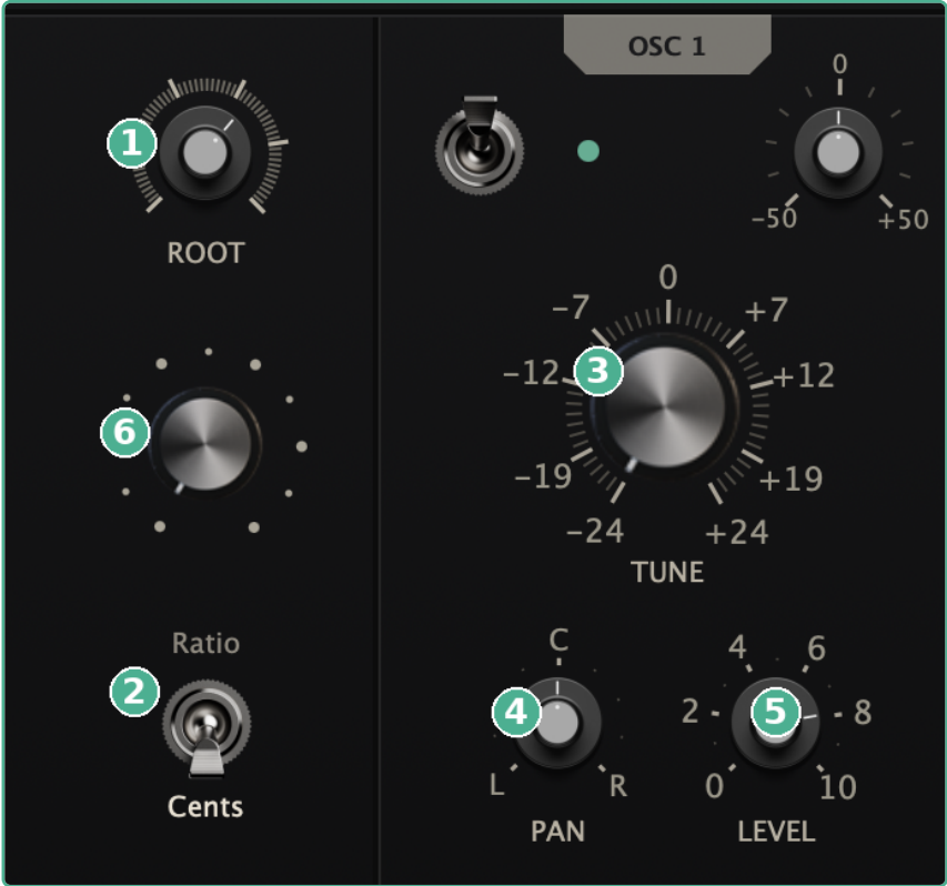
A DRONE oscillator: ① Root (shared fundamental) · ② Ratio/Cents mode · ③ Tune (degree or offset) · ④ Pan · ⑤ Level · ⑥ Cluster (squeezes or spreads the pitches).
