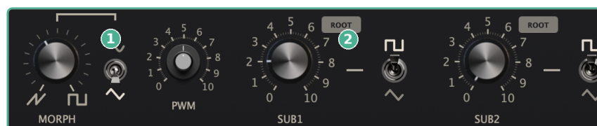
Two details of the VOICE row: ① the TRI / SIN switch at the centre of the morph · ② the ROOT button (on each sub) that locks the oscillator to the drone fundamental.
