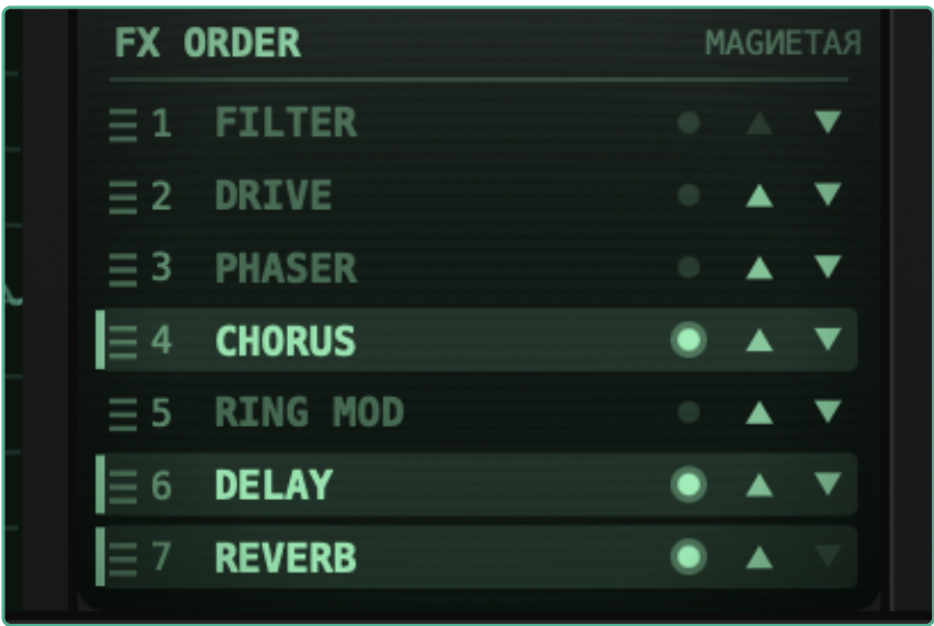
The FX ORDER screen: the seven modules in their processing order, with active (ON) effects highlighted in green with their LED.
