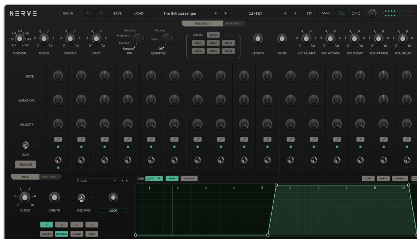
The SEQUENCE 2 screen: the 16-step sequencer (top) and the four drawable MSEG envelopes (bottom).
